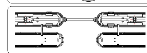
**STEP 7:** Install the diffuser to the waterproof fitting and close the clips.
