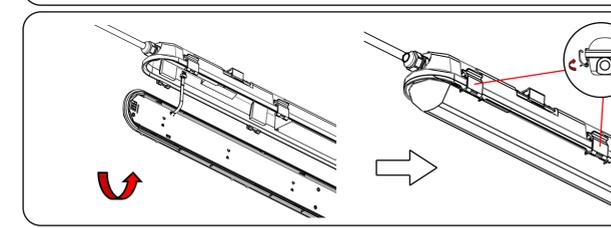
**STEP 7:** Wire the waterproof fitting to the main power supply. Ensure to use waterproof terminal block [not included].
